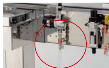
Type NTW: Rear view Ejector installed.
